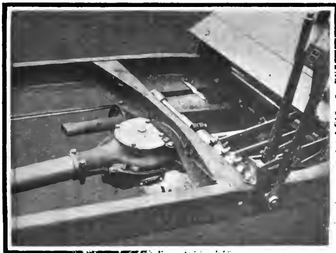
Gearbox on front end of torque tube, Bianchi light car
